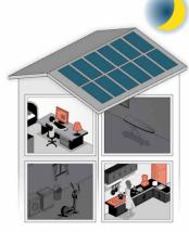
**Nighttime:** Important loads are powered by the battery
