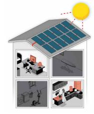
**Daytime:** Important loads are powered first by the PV system and then by the battery. The battery can be charged from the PV as needed
