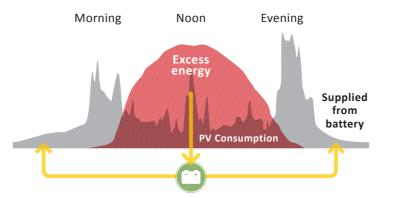
Using StorEdge, excess energy produced during peak sunlight hours when consumption is low is stored to a battery and used later. Energy isn't wasted!
