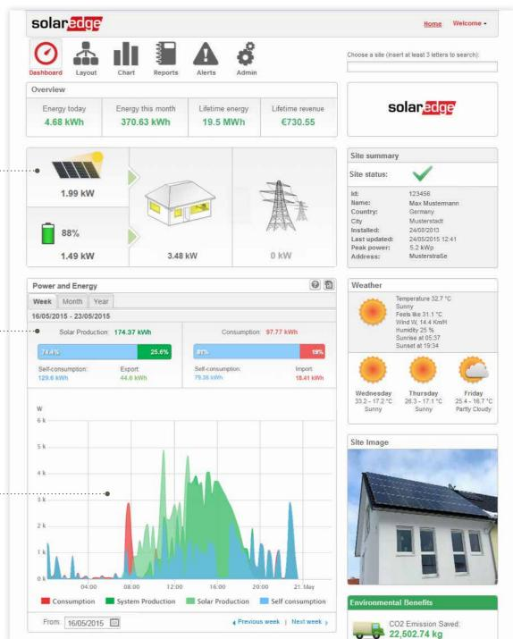
Dashboard from the SolarEdge cloud-based monitoring platform
